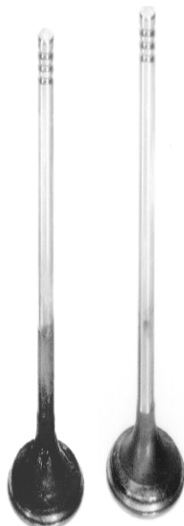
Figure 11: Inlet valves after representative engine tests with the base petrol fuel ( left ) and membrane treated fuel (i.e. the permeate, right ).
